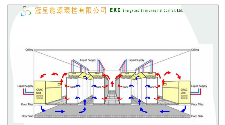
Figure 13. Local cooling distribution using overhead cooling units mounted to the ceiling.
