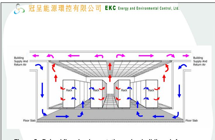
Figure 5. Raised floor implementation using building air from a central plant.
