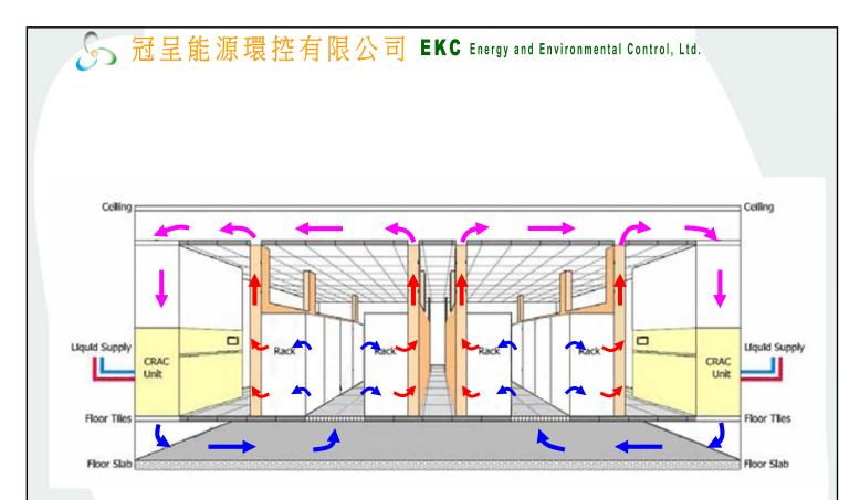
Figure 11. Raised floor implementation using outlet plenums / ducts integral to the rack.
