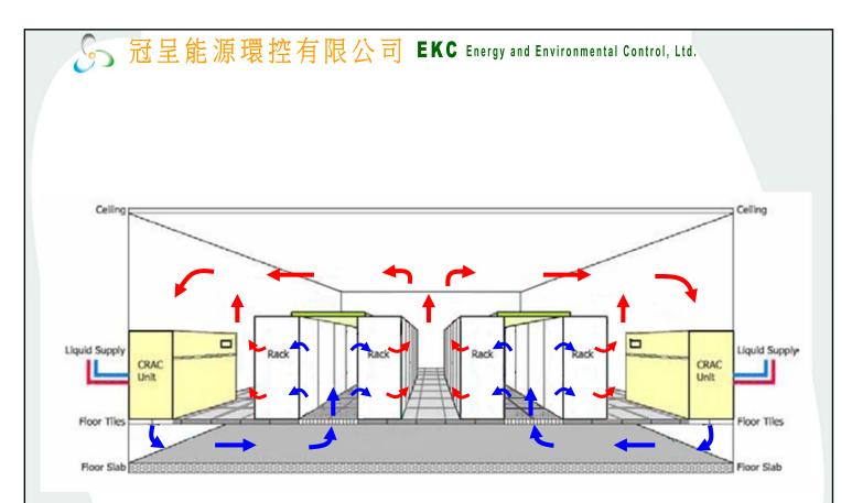
Figure 9. Raised floor implementation using baffles to limit hotaisle/cold-aisle "mixing".
