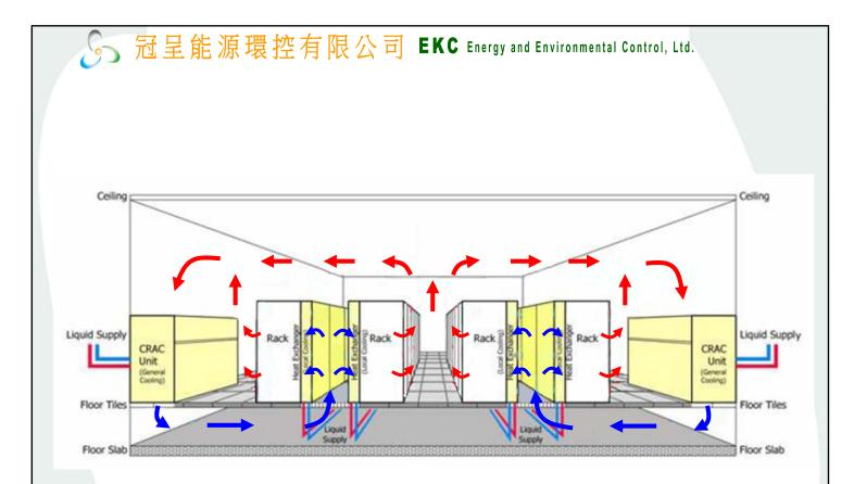
Figure 15. Local cooling via integral rack cooling units on the inlet side of the rack.
