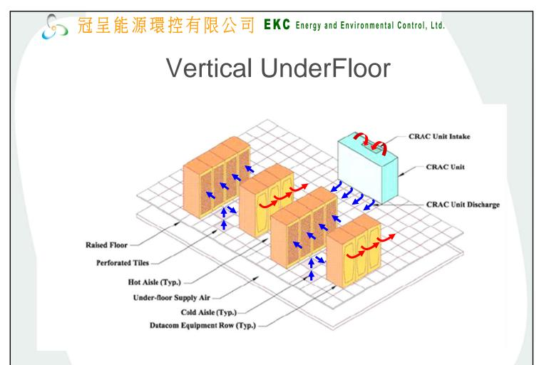
Figure 1 Example data contor with VIIE cooling architecture
